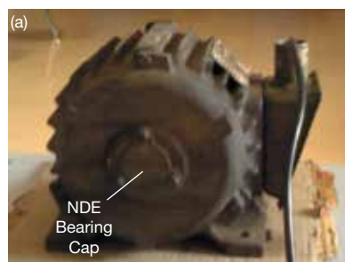
▲ Figure 3. An external temperature rise at the nondrive end (NDE) bearing cap of a motor (a) can be detected by comparing normal (b) and abnormal (c) thermographic images. Temperature changes could indicate a problem.
