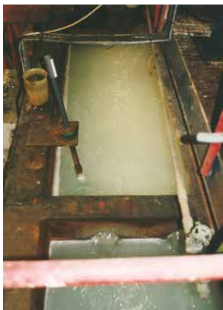
▲ Figure 3. Large pH dosing tanks may be the source of inefficient pH control.
